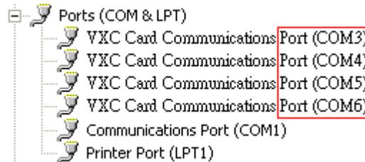
This problem usually occurs because COM1 and COM2 are set to be used by the operating system itself, meaning that you will not be able to use either of these COM Ports unless the current functions are stopped beforehand. To resolve this issue, follow the process described below to complete configuration.
